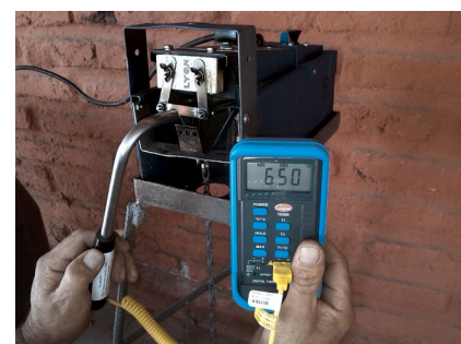
Pyrometer indicating proper blade temperature of 650°C.
